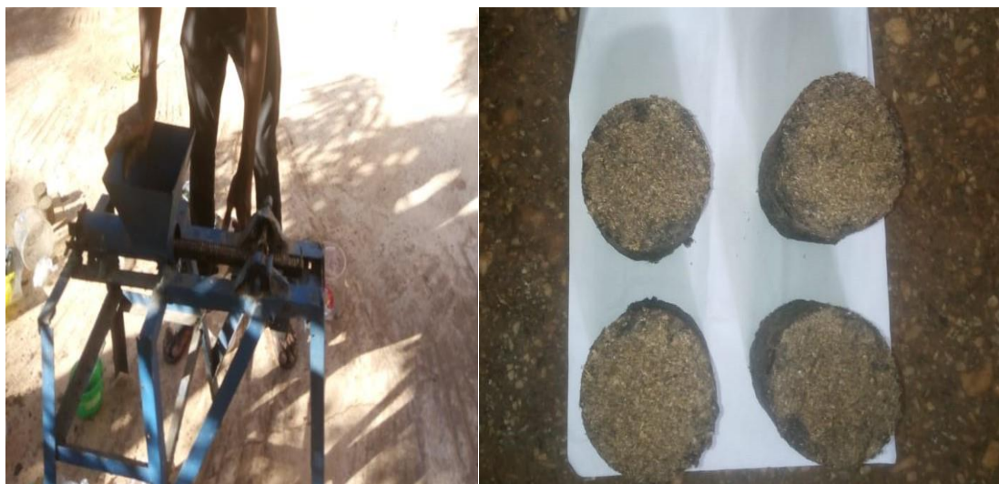
Figure 1. Image of homemade fabricated briquetting machine and produced briquette
